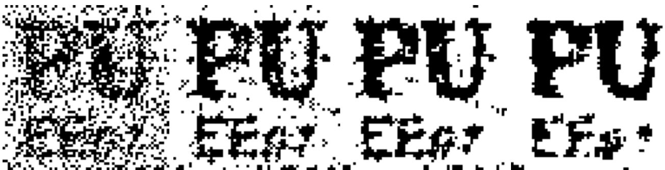
Figure 6. Extracted watermark images from 512 \times 512 watermarked “Baboon” with JPEG compression with quality factor of 15% for (from left to right) Case 1, Case 2, Case 3 and Case 4.
