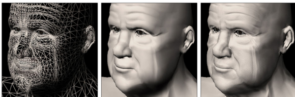
Figure 2: Wireframe, normal mapped and additionally bump mapped
