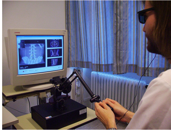
Figure 2. Trainee using the virtual lumbar puncture trainer using stereographic visualization with shutter glasses.
