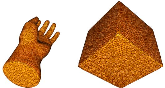
**Figure 11:** Discontinuity modeling provides for mesh edges which map to the object edges.
