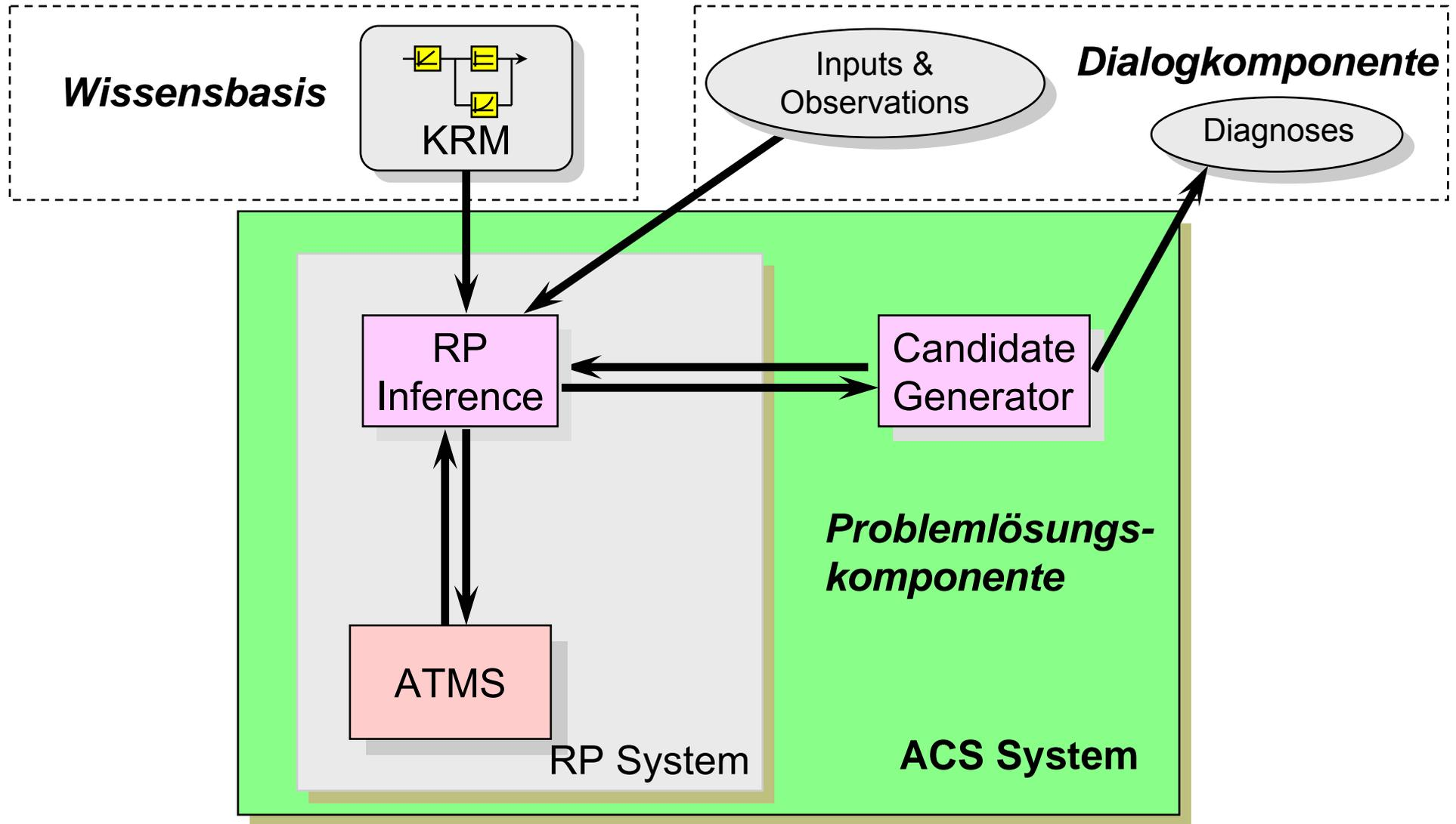
**ACS: Assumption-based Constraint Solver**
